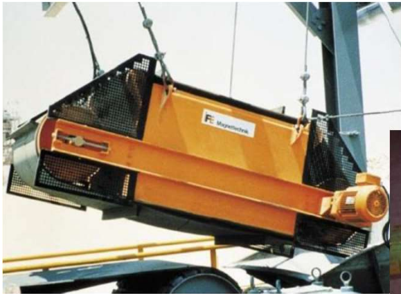
Figure 9 Overband magnet (used to separate larger ferro parts)
