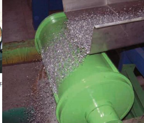
Figure 10 Drum magnet (used to separate small sizes ferro parts)
